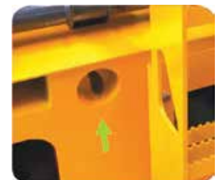
Emergency Drop Valve
